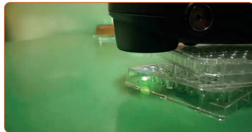
Figure 6: Experimental set-up: cross-linking the bacterial solutions.
